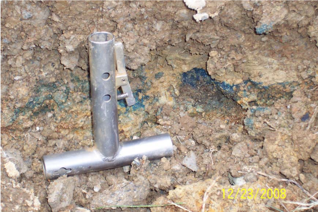
Photo 3 - Impacted "green" soil on western side of vault excavation to north of Building 41.
